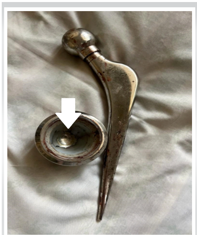
Figure 3: Implants after removal showing polyethylene liner wear in the cup (marked by arrow) and the femoral stem.
