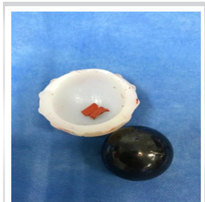
Figure 2: The two particles – measuring 3 \times 1 \times 8 mm – originating from the trial femoral head implant with the scratched polyethylene liner.
