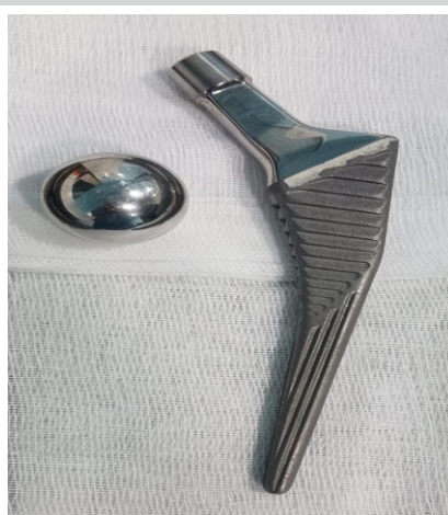
Figure 4: Explanted stem demonstrated the absence of hydroxyapatite coating.
