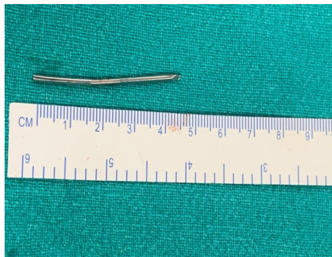
Figure 6: Showing removed broken k-wire of 45–50 mm length found slightly bent at the center.
