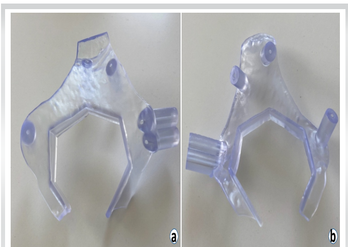
Figure 6: (a) Cutting guide in BioMed clear after printing. (b) Cutting guide in BioMed Clear after printing.
