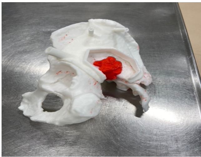
Figure 7: Picture of the printed model (tumor in red) and the first iteration of the cutting guide.
