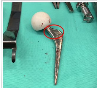
Figure 2: Demonstrating fractured retrieved V40 Exeter stem
