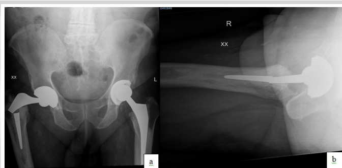
Figure 1: (a and b) AP and Lateral radiographs showing a fracture through proximal and middle third of V40 Exeter stem.
