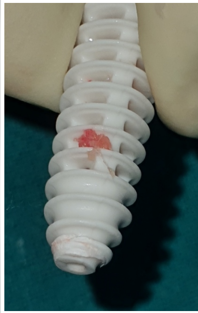
Figure 2: Flattening of screw thread.
