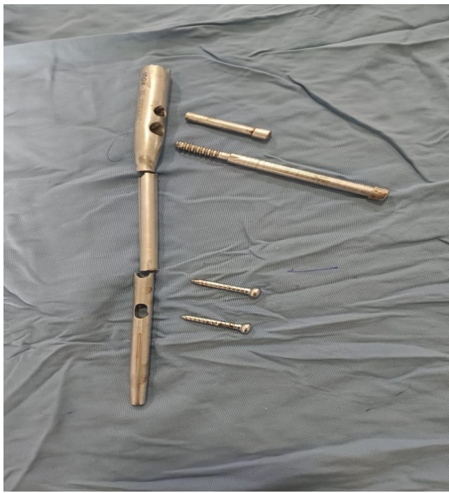
Figure 7: Image illustrating the extracted implant showing the nail broken at two sites and the broken proximal screw.
