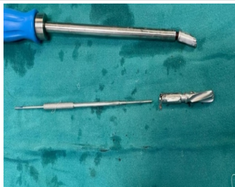
Figure 5: Screwdriver removed the broken piece of the PFNA- II blade.
