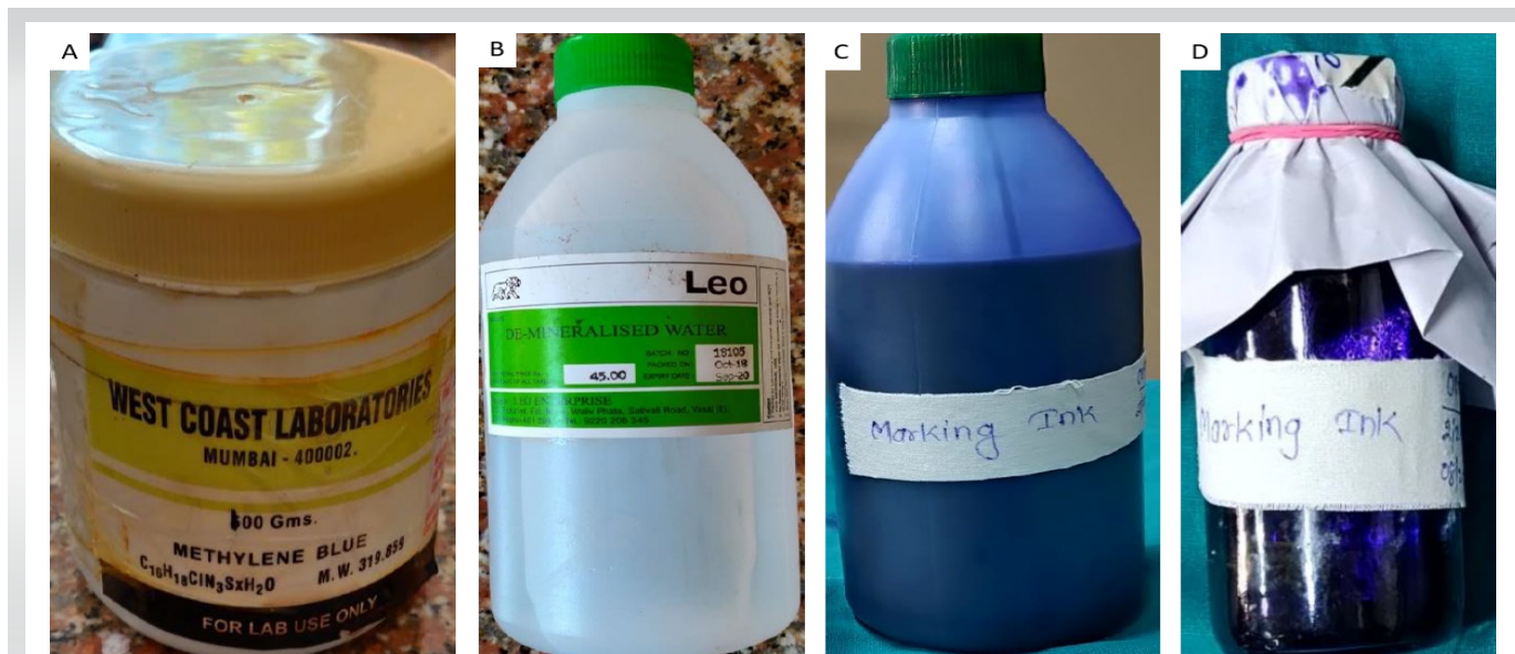
Figure 1: Preparation of ink (A) Methylene blue powder, (B) Demineralized water, (C) Prepared ink, (D) Autoclavable glass bottle for sterilization.
