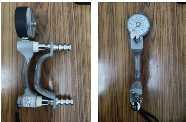
Figure 1: Hand dynamometer is used to measure the static hip abductor strength assessment. Dynamometer was calibrated before assessing every patient.
