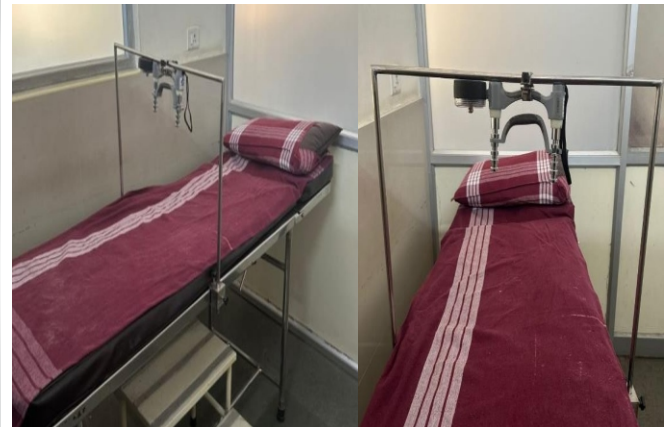
Figure 2: Dynamometer was fixed in solid bar to check for static hip abductor strength.
