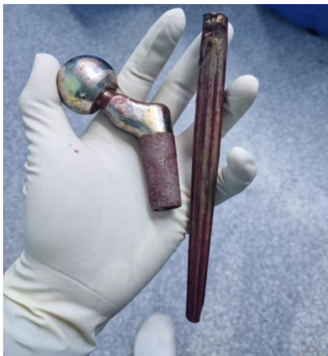
Figure 4: Clinical photograph showing the failed Zimmer modular revision stem.
