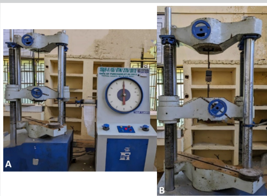
Figure 2: Universal testing machine setup used for axial pull-out testing, showing (a) the overall testing apparatus and (b) the cement–screw construct mounted and aligned for application of axial tensile load.
