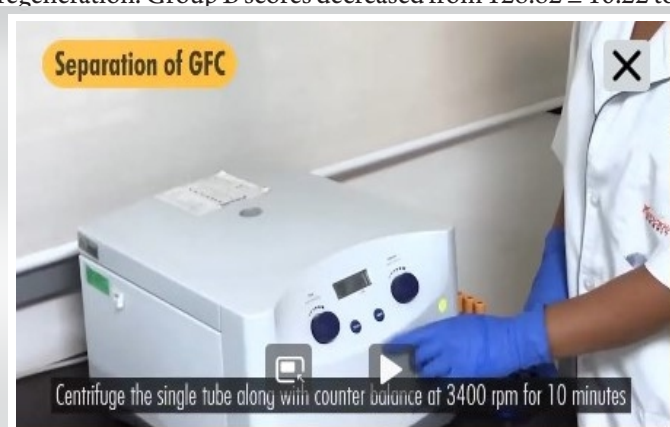
Figure 3: Step 3 of preparation of GFC
