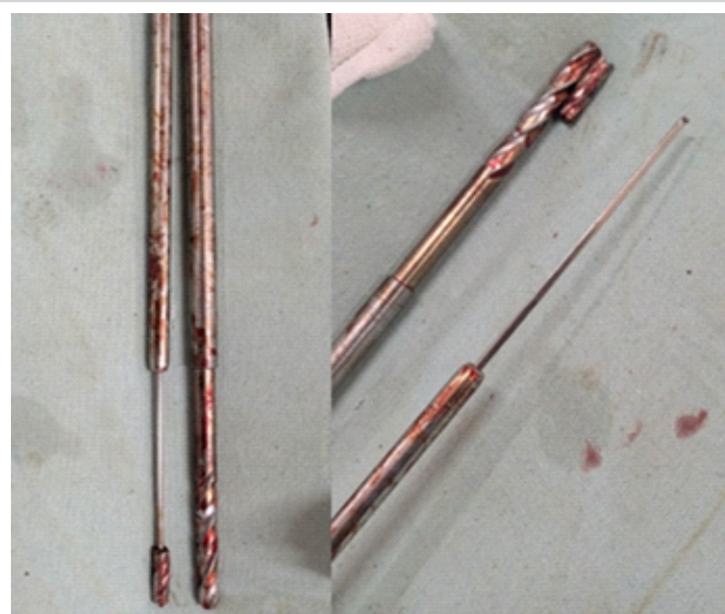
Figure 4: Intraoperative picture of broken drill bit post-retrieval. Intraoperative photograph demonstrating the retrieved broken 8-mm cannulated drill bit alongside the depth gauge used for its extraction. The intact cannulated drill bit is shown for comparison.
